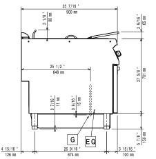
EQ = Equipotential screwG = Gas connection
